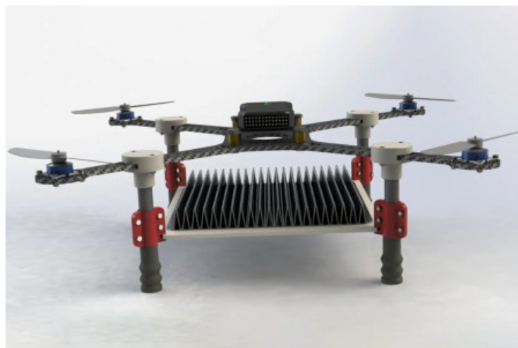
Figura 16. Dron alimentado mediante un láser [Northwestern Polytechnical University].
