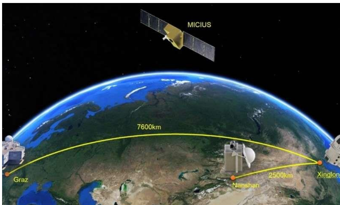
Figure 6. Diagram of the network established for this long-distance communication. (Phys.org, (2018))
