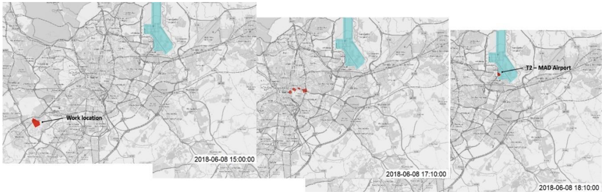
Fig. 4. Example of the use of mobile phone records to identify a departing passenger and their potential activity and coarse trajectory to the airport (additional intermediate locations are omitted in this sequence).
