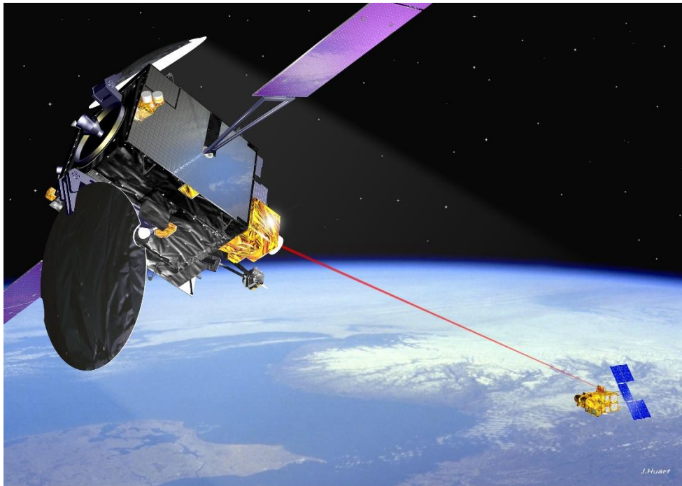
Figure 15: ESA world demonstration the first laser link between Artemis and SPOT4 on 22 nd November 2001 communicating via SILEX.
