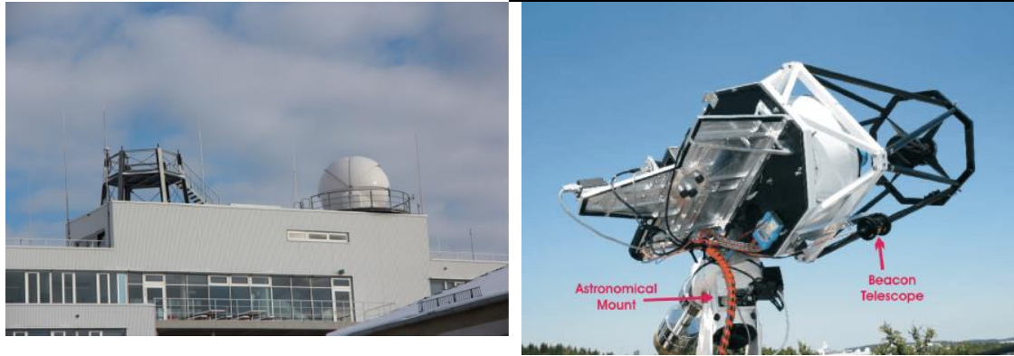
Figure 11: (a) DLR Optical Ground Station (OGS) dome at Oberpfaffenhofen, and (b) View of the focal bench of the 40-cm telescope.
